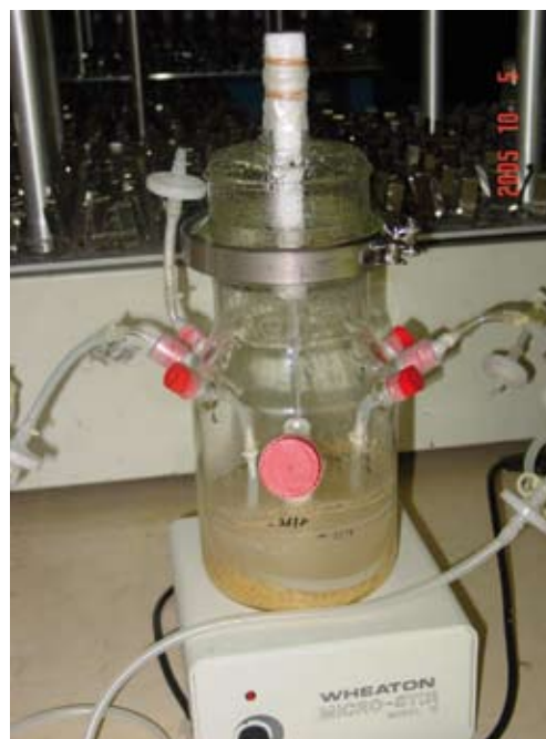
Figure 1. MPOB Modified Vessel (MoVess) for liquid tissue culture system.
