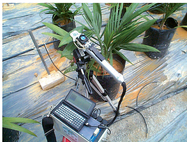
Figure 1. Gas exchange measurement on oil palm seedling.
