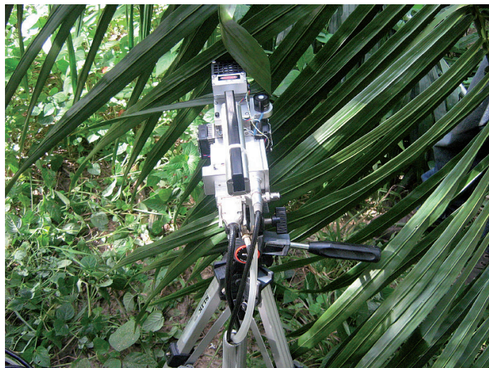
Figure 2. Gas exchange measurement on six-year-old palm.
