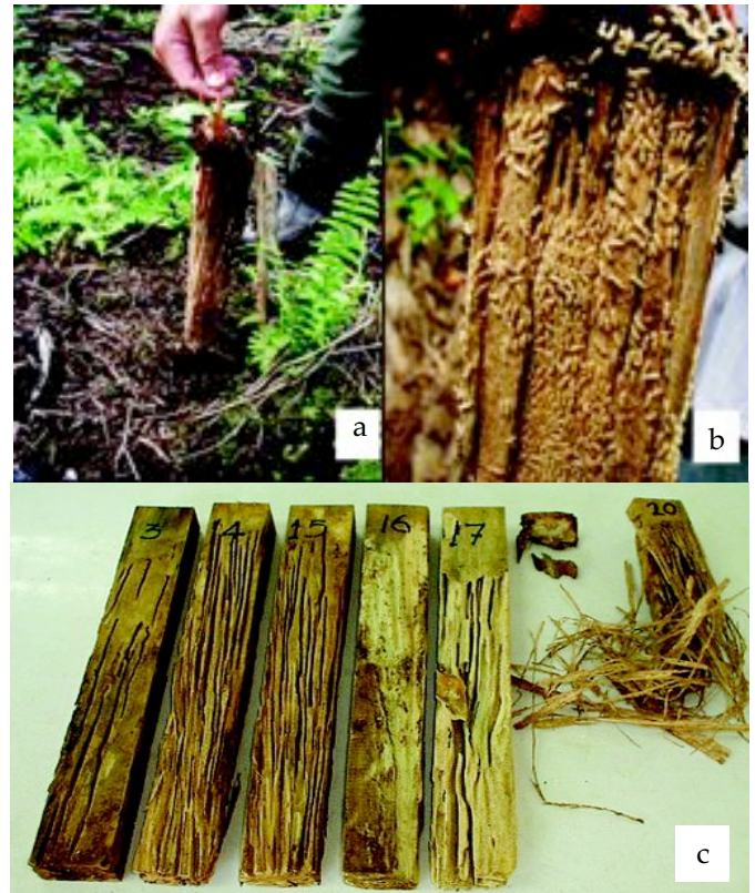
Figure 4. Rubstake infested with termites after one month in peat soil (a), workers of C. curvignathus on Rubstakes (b) and damage on Rubstakes by C. curvignathus (c).
