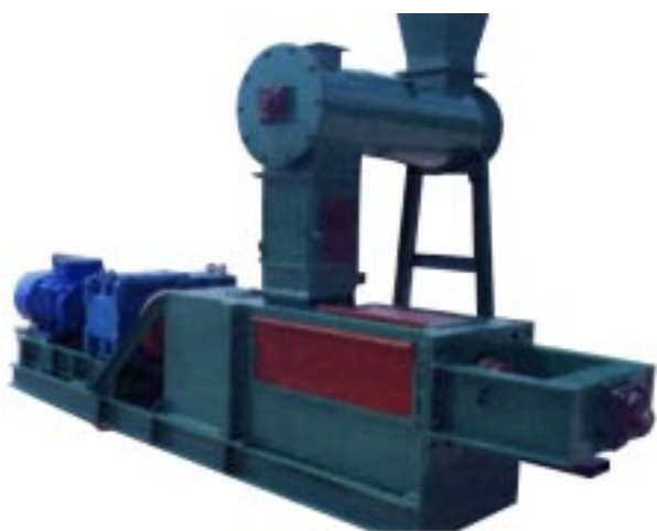
Figure 1. Hammer mill and water cooled screw press.
