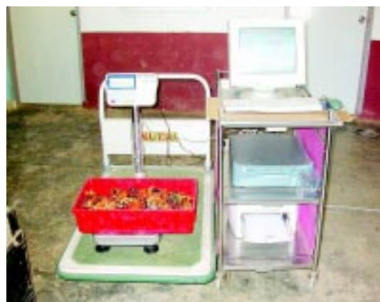
Direct data capturing system where data are automatically captured into the computer and the error-free data can instantly be retrieved.
