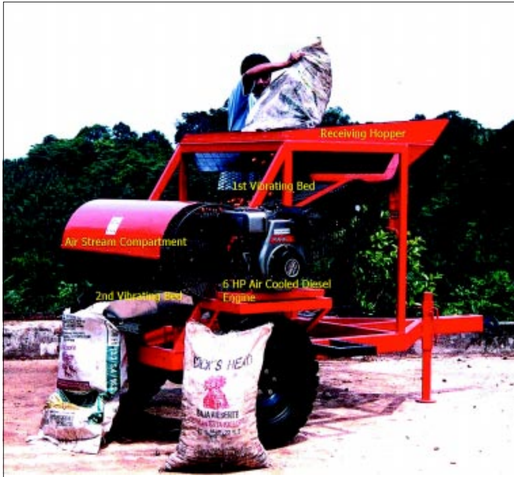
Figure 1. Fruits from fertilizer bags are emptied onto the receiving hopper and with the help of vibration mechanism and air stream, the clean fruits are collected just after the second bed.
