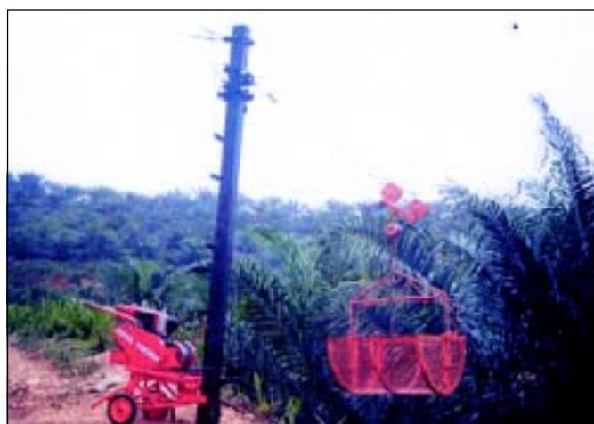
Figure 1. The cableway system: pylon, power unit, chain block and bucket.
