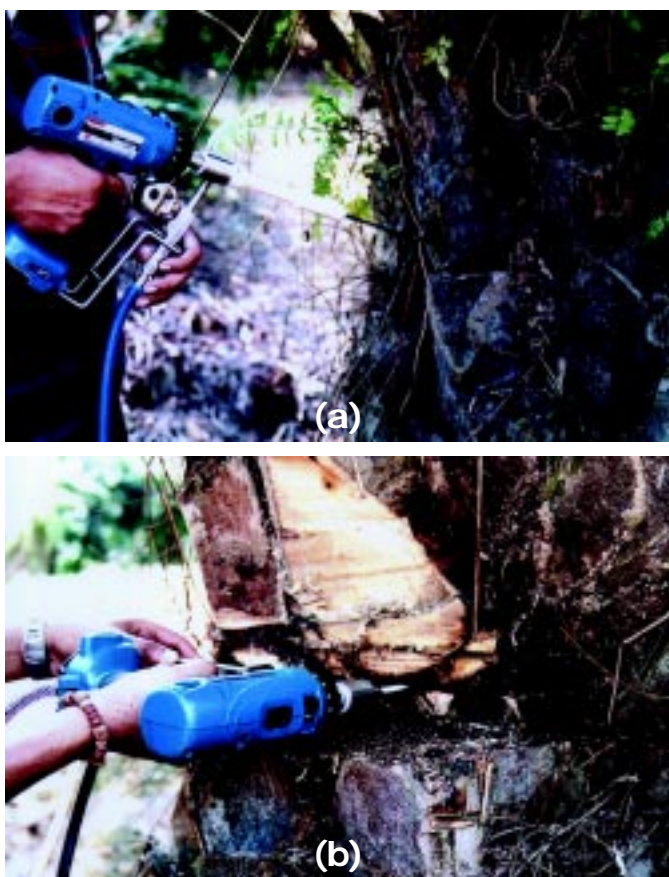
Figure 3. (a) Drilling palm trunk to make a hole before putting the injector (b) injecting dye into the trunk.
