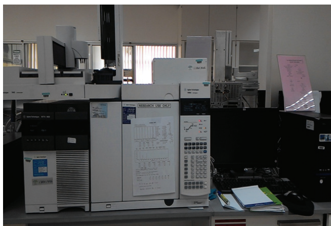
Figure 4. Gas-chromatography-mass spectrometer detector for determination of dimethyl sulfate in palm-based methyl ester sulfonate.
