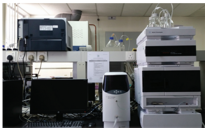
Figure 2. High Performance Liquid Chromatography (HPLC) – Size Exclusion Chromatography with Evaporative Light Scattering Detector (ELSD) for the quantification of polar compound fractions.
