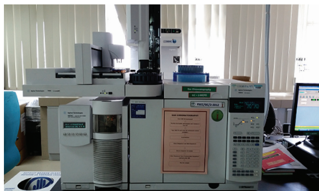
Figure 2. GC-MS instrument for the analyses of 2- and 3-MCPD esters and GE in oils and fats.
