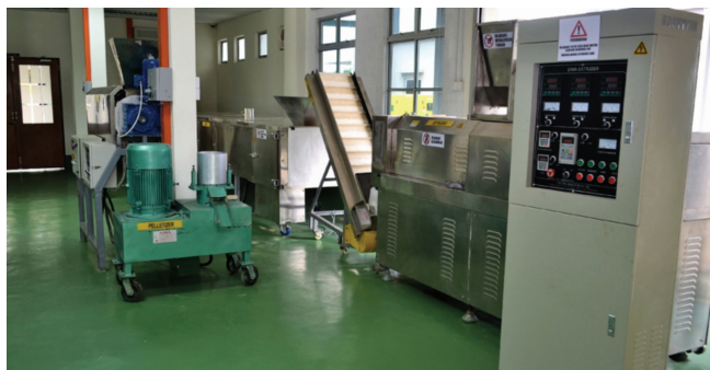
Figure 3. A 100 kg hr -1 MPOB Animal Feed Pilot Plant at MPOB Keratong Research Station, Pahang.
