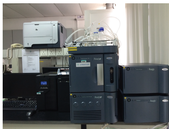
Figure 1. UPLC-RID for TAG determination in palm oil products.
