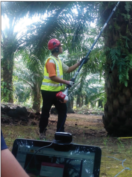
Figure 3. Vibration test during cutting (left) and Dewesoft vibration equipment (right).
