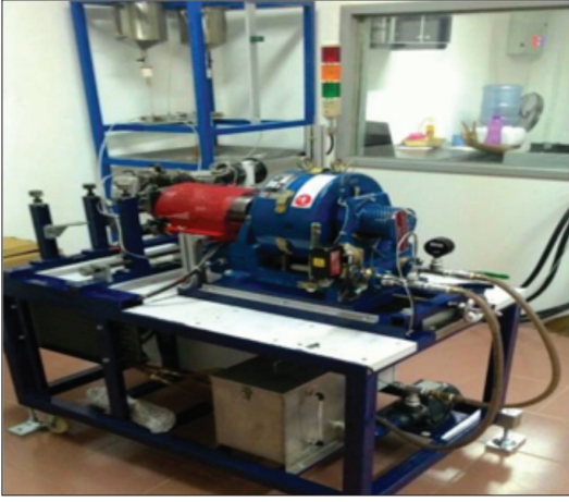
Figure 5. Engine dyno for engine's performance and endurance test (left) and control room (right).
