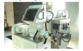
Compress the homogenised soap using a large worm screw extruder or plodder. A single large continuous bar of soap is produced and the dimension is adjusted to fit the size of the final product with minimum waste.
