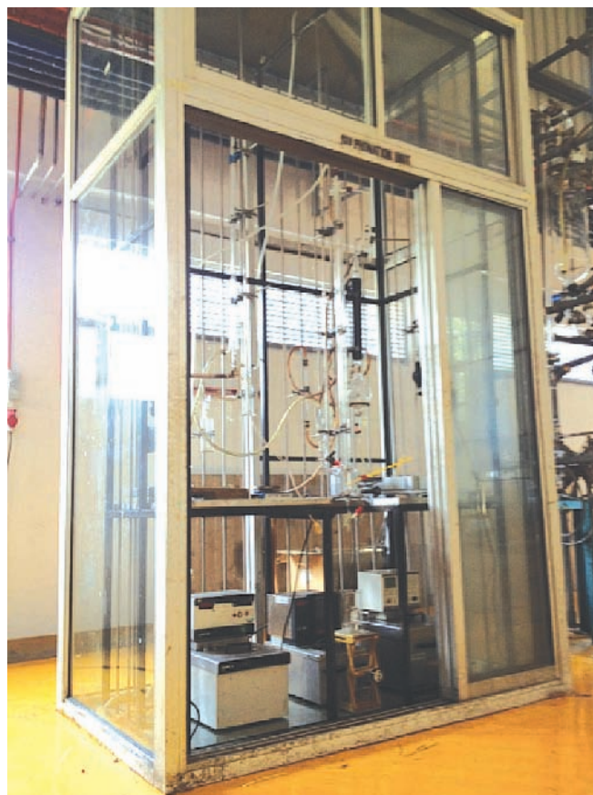
Figure 3. Mini sulphonation pilot plant of 600 g hr -1 production capacity.
