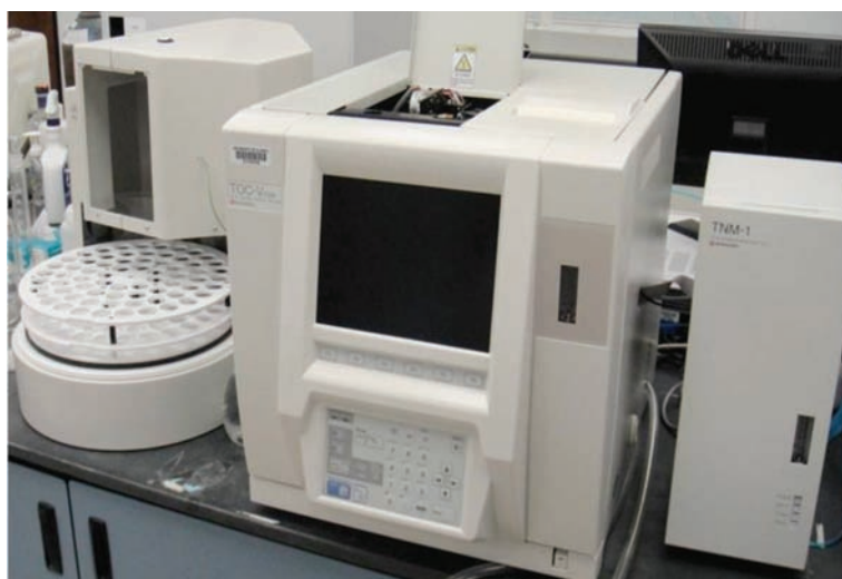
Figure 1. The instrument used to determine total carbon (TC), total nitrogen (TN), total organic carbon (TOC) and carbon per nitrogen (C/N) (TOC-VCPN and TN -1, Shimadzu Japan).
