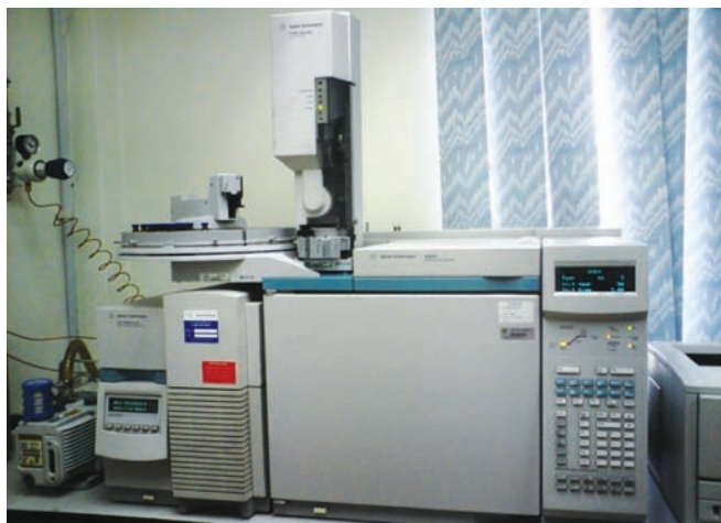
Figure 2. Gas chromatography-mass spectrometry (GC-MS) for volatile organic compound (VOC) analysis.
