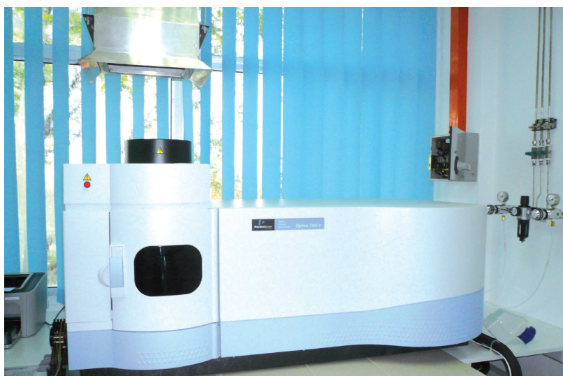
Figure 1. Inductively coupled plasma optical emission spectrometer (ICP OES).
