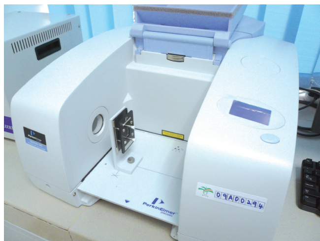
Figure 1. Fourier transform infrared (FTIR) spectrometer with a CaF 2 sample cell.
