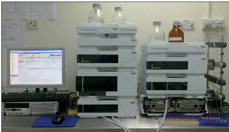
Figure 2. High performance liquid chromatography (HPLC) instrumentation system for the donor-acceptor complex chromatography (DACC) method.
