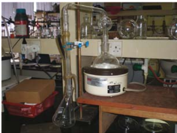
Figure 4. Apparatus set-up for determination of ammoniacal nitrogen.
