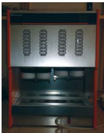
Figure 6. Soxhlet extraction unit for determination of oil and grease.
