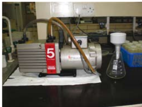
Figure 5. Apparatus set-up for determination of suspended solids.
