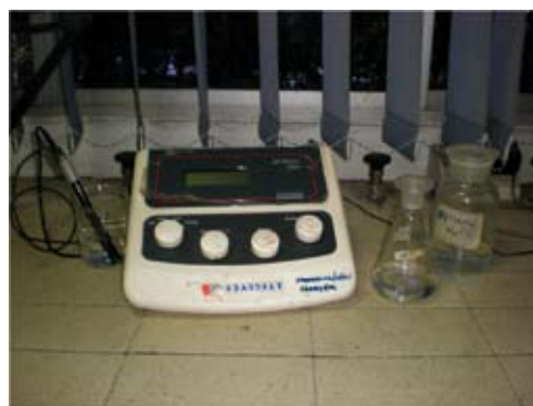
Figure 8. pH meter for determination of total alkalinity.
