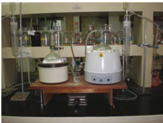
Figure 3. Micro-Kjeldhal digestion and Hoskin's distillation apparatus for determination of total nitrogen.
