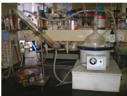
Figure 7. Markham's still distillation apparatus for determination of volatile fatty acids.
