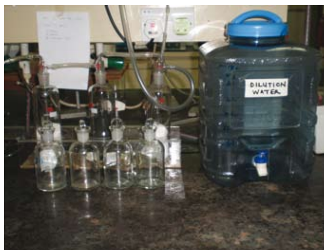
Figure 1. Apparatus set-up for determination of BOD.
