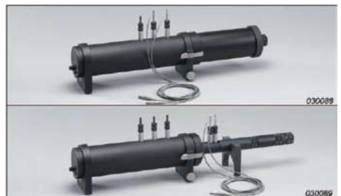
Figure 2. Type 4206 impedance tube standard large (above) and small (below) set-ups.
