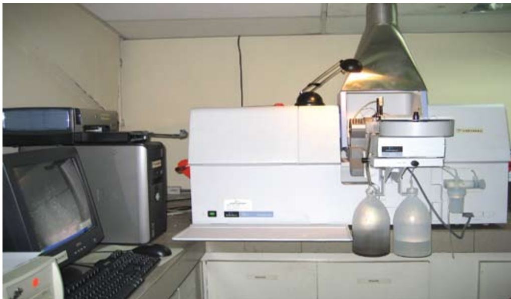
Figure 1. Graphite furnace atomic absorption spectrometer for determination of \text{TiO}_2 in soap noodles.
