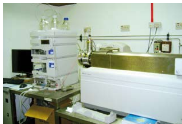
Figure 2. High performance liquid chromatography with MS/MS detector.
