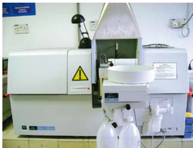
Figure 2. Graphite Furnace Atomic Absorption Spectrometry for determination of arsenic in palm kernel cake.
