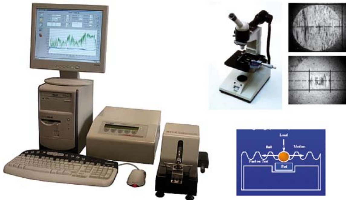
Figure 1. High frequency reciprocating rig (HFRR) test system.
