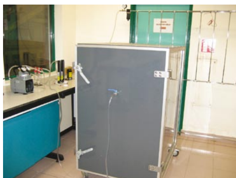
Figure 1. Formaldehyde emission test chamber.
