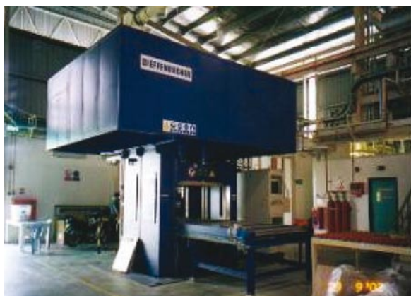
Figure 2. Hot press for panel preparation.
