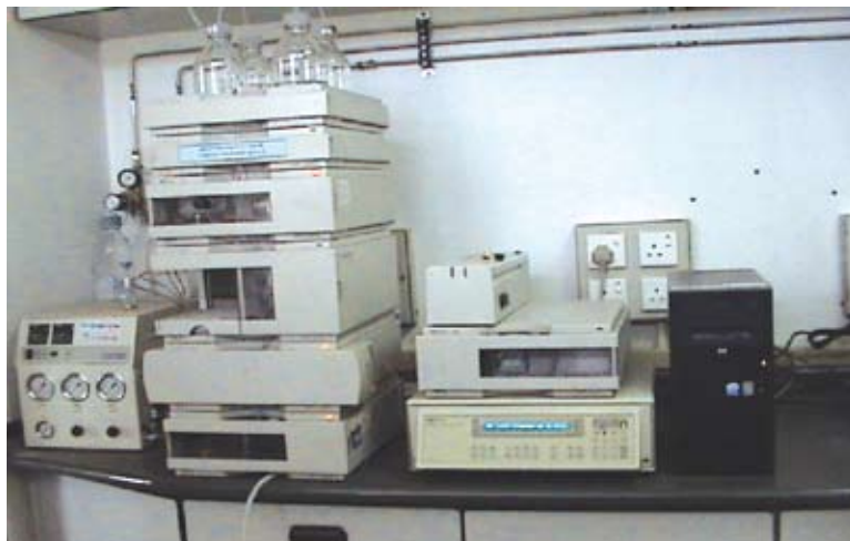
Figure 3. HPLC for fluroxypyr analysis.
