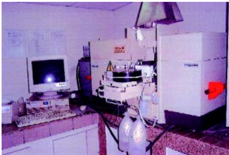
Figure 1. Graphite furnace atomic absorption spectrometer for the detection of arsenic in edible oils.
