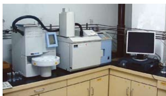
Figure 1. Gas chromatography for determination of glycerides, free and total glycerol, methanol and esters contents.
