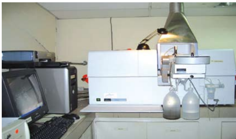
Figure 1. Graphite furnace atomic absorption spectrometer for determination of arsenic in glycerine.
