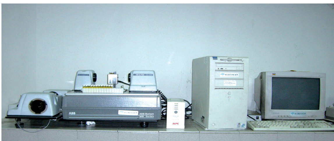
Figure 1. Near infra-red (NIR) spectroscopy equipment for determination of oil residue in methyl esters.
