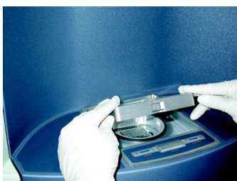
Figure 5. Loading the sample into MALDI-TOF MS.
