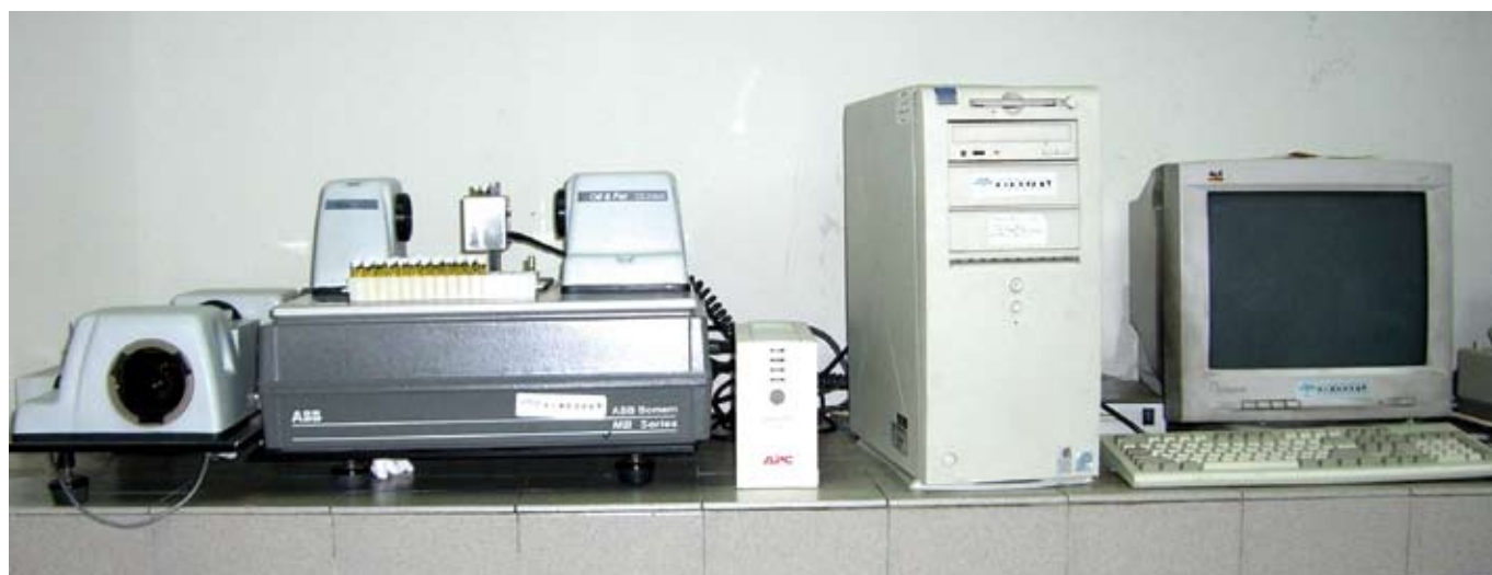
Figure 1. Near infra-red spectroscopy for determination of alcohol bottom and ester bottom in CPKO.
