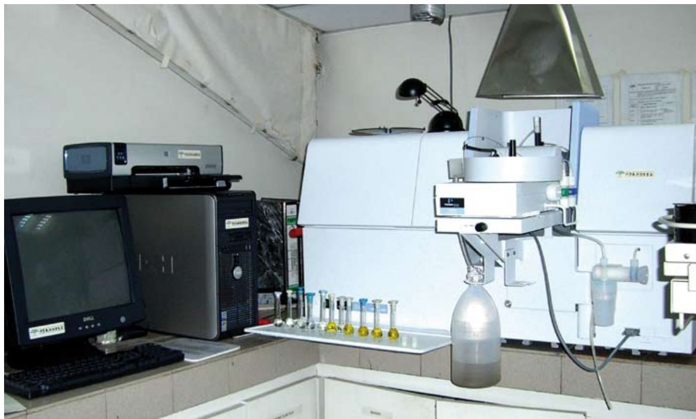
Figure 1. Graphite furnace atomic absorption spectrometer for the detection of titanium (organic) in fatty acids.
