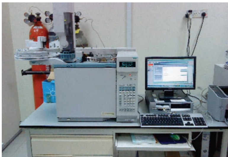
Figure 1. Gas chromatography with flame ionisation detector instrument.
