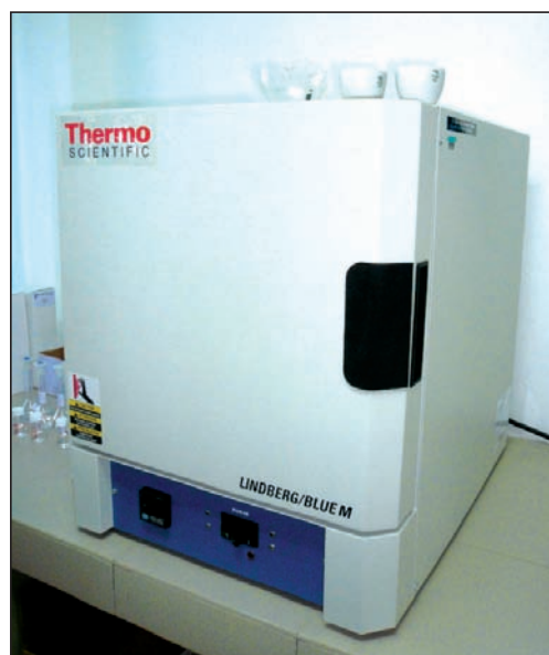
Figure 1. Furnace and evaporating dish.
