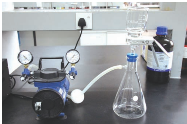
Figure 2. Membrane filter system.
