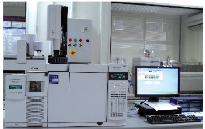
Figure 2. Gas chromatography with a mass selective detector (GC-MSD) instrumentation system.
