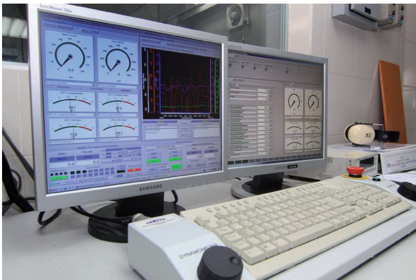
Figure 2. Fully computerised control of the dyno operation.
