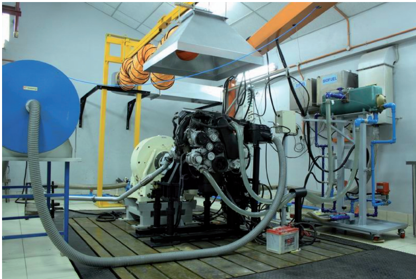
Figure 1. Engine dynamometer facility setup.
