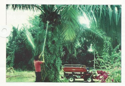
The mechanical cutter is attached to an infield transporter that carries the harvested FFB. This cutter is suitable for cutting and pruning.
