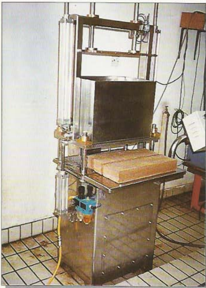
Figure 2. Prototype Moulding Machine for Planting Medium from Oil Palm Biomass
