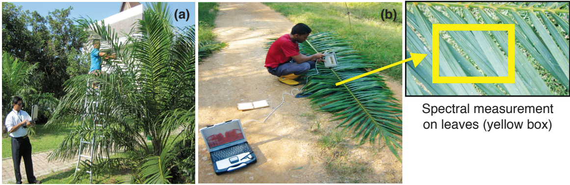
Figure 2. Data measurement using a field spectroscopy on (a) immature young and (b) mature oil palm.
